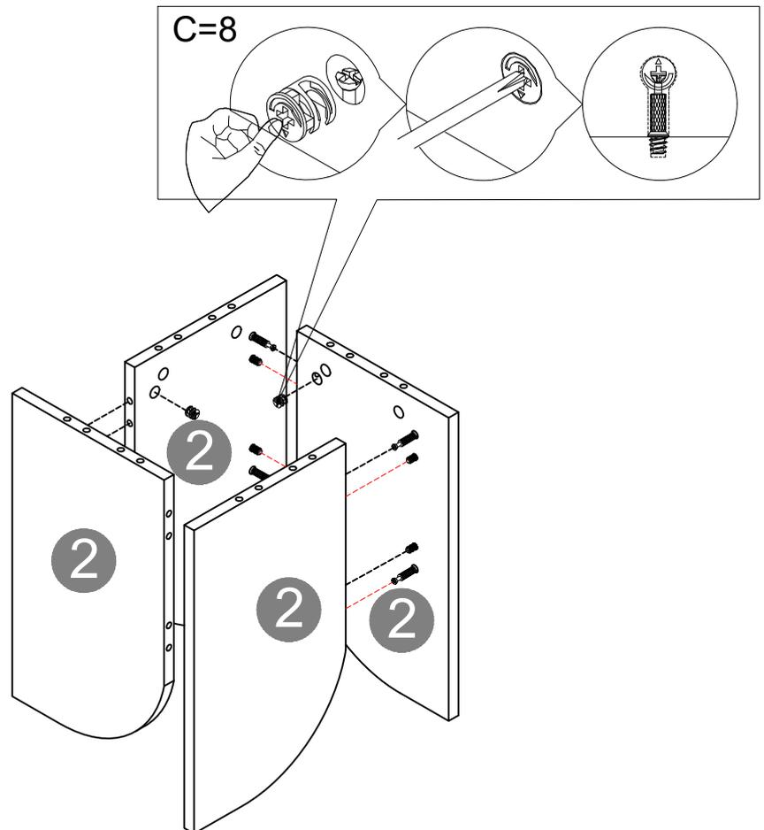
STEP 3: Fix panel (1) to panel (2) with cam lock (C).
